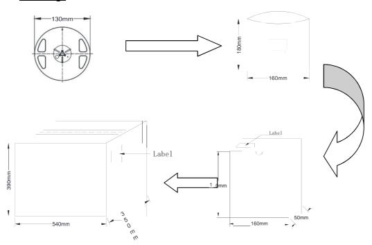
Note:5 meters/reel, 1reel/antistatic bag, 3 antistatic bags/box, 20 box/export carton;
